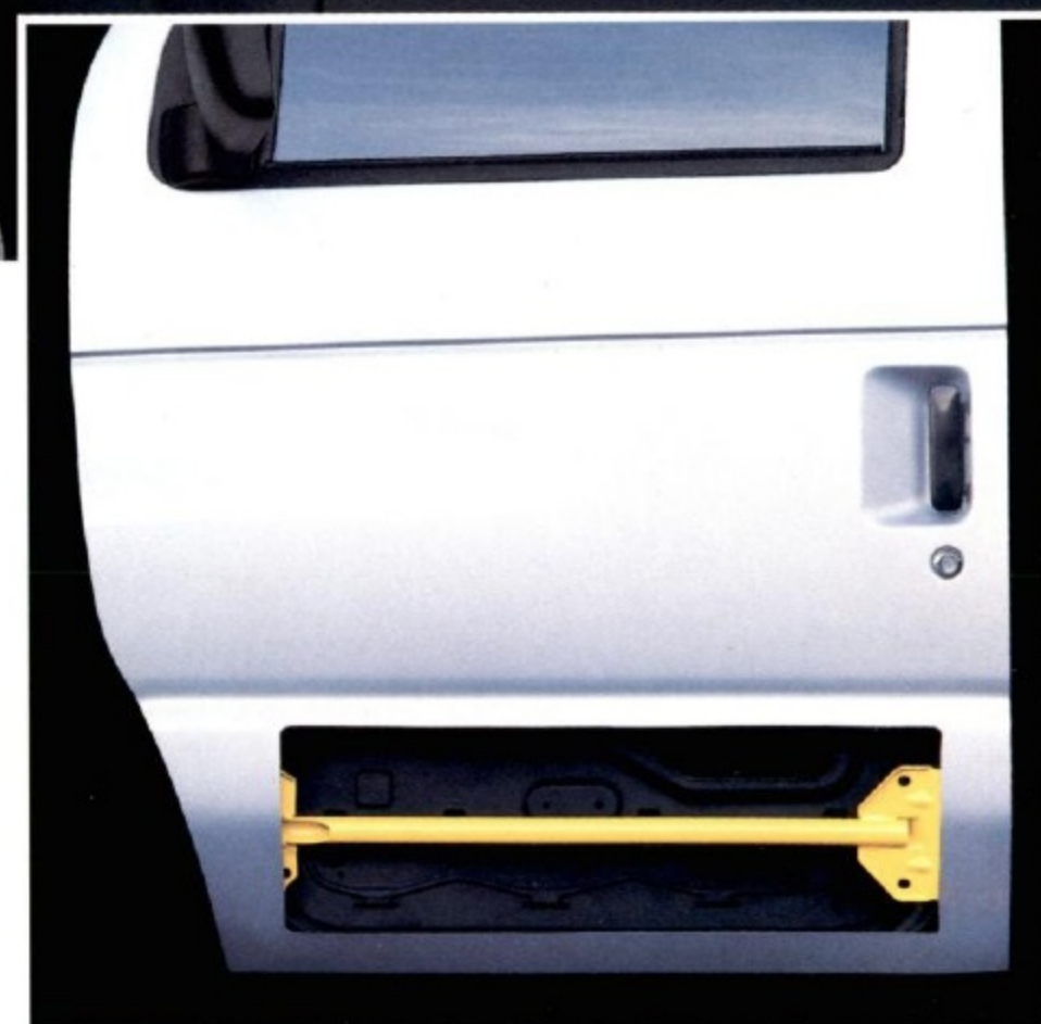
Side door intrusion beams are integral components of Econoline's strong occupant protection system.
