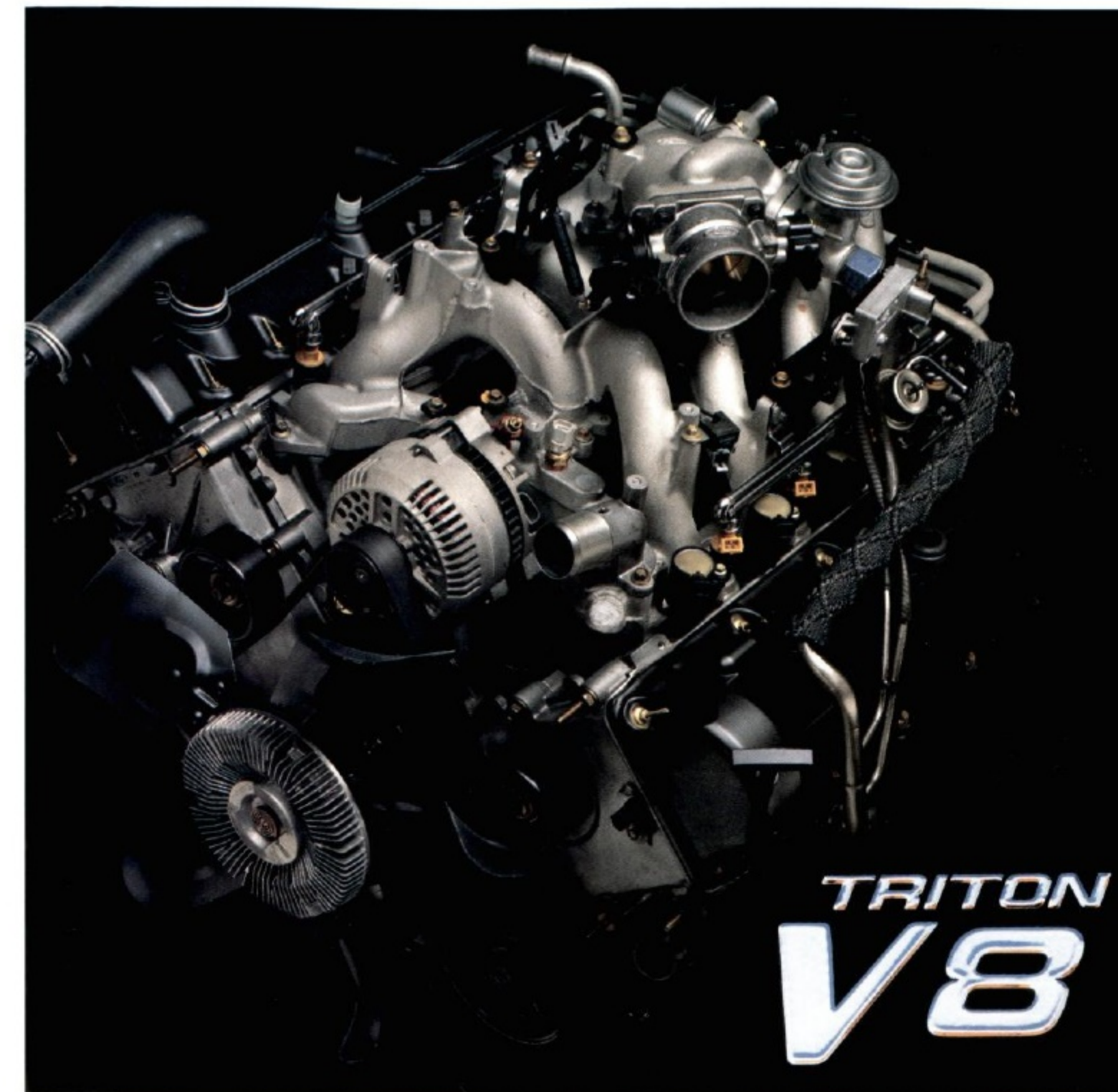
The 5.4L Triton V8 has a raised deck and a longer stroke than the 4.6L V8 for higher performance. Like the 4.6L, the 5.4L features a chain-driven single overhead camshaft (SOHC) and a specially tuned aluminum upper and lower intake manifold assembly designed for low-rpm/high-torque applications like trailer towing. Cargo haulers especially will appreciate the way this engine's low-end torque can get their heavy loads underway powerfully and smoothly.
