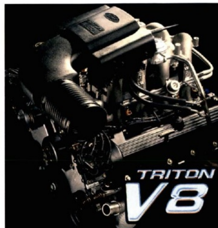
The 4.6L Triton V8, with chain-driven single overhead cam (SOHC) design, delivers more horsepower per liter of displacement over the engine that preceded it. Low-end torque performance is excellent, thanks to a specially tuned induction system.
