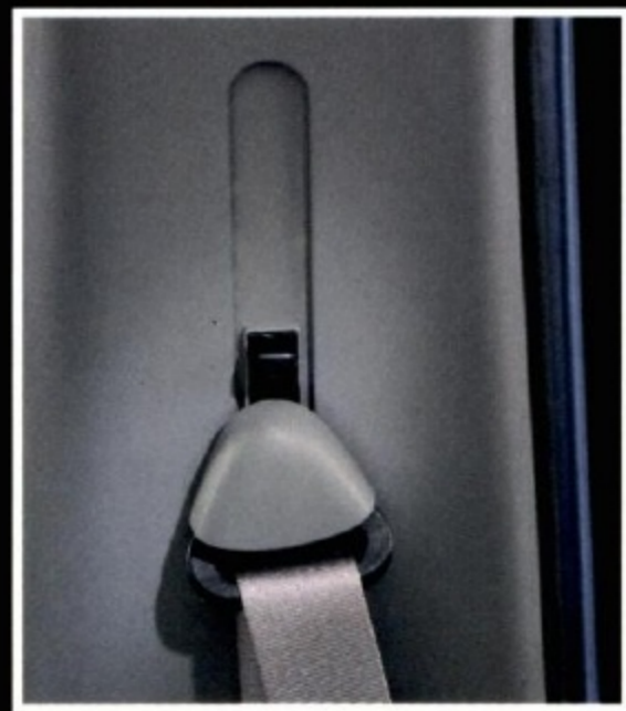
Front seat shoulder belts are height-adjustable for individual comfort.
