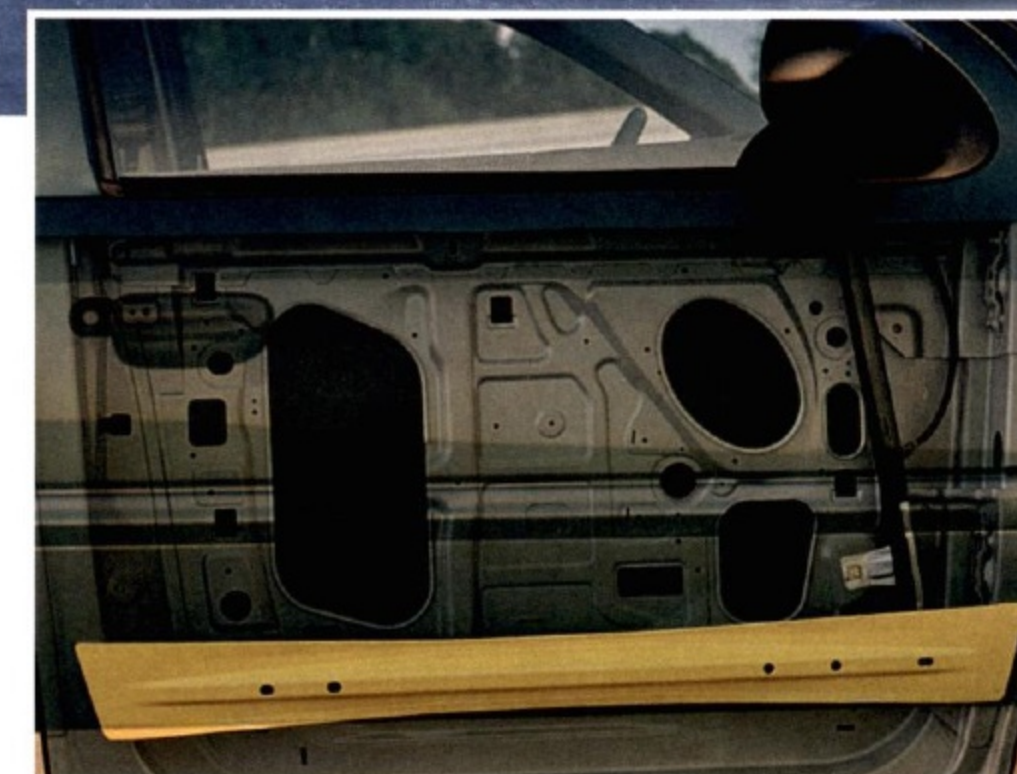
Side door intrusion beams are just one of a long list of Windstar safety features.
