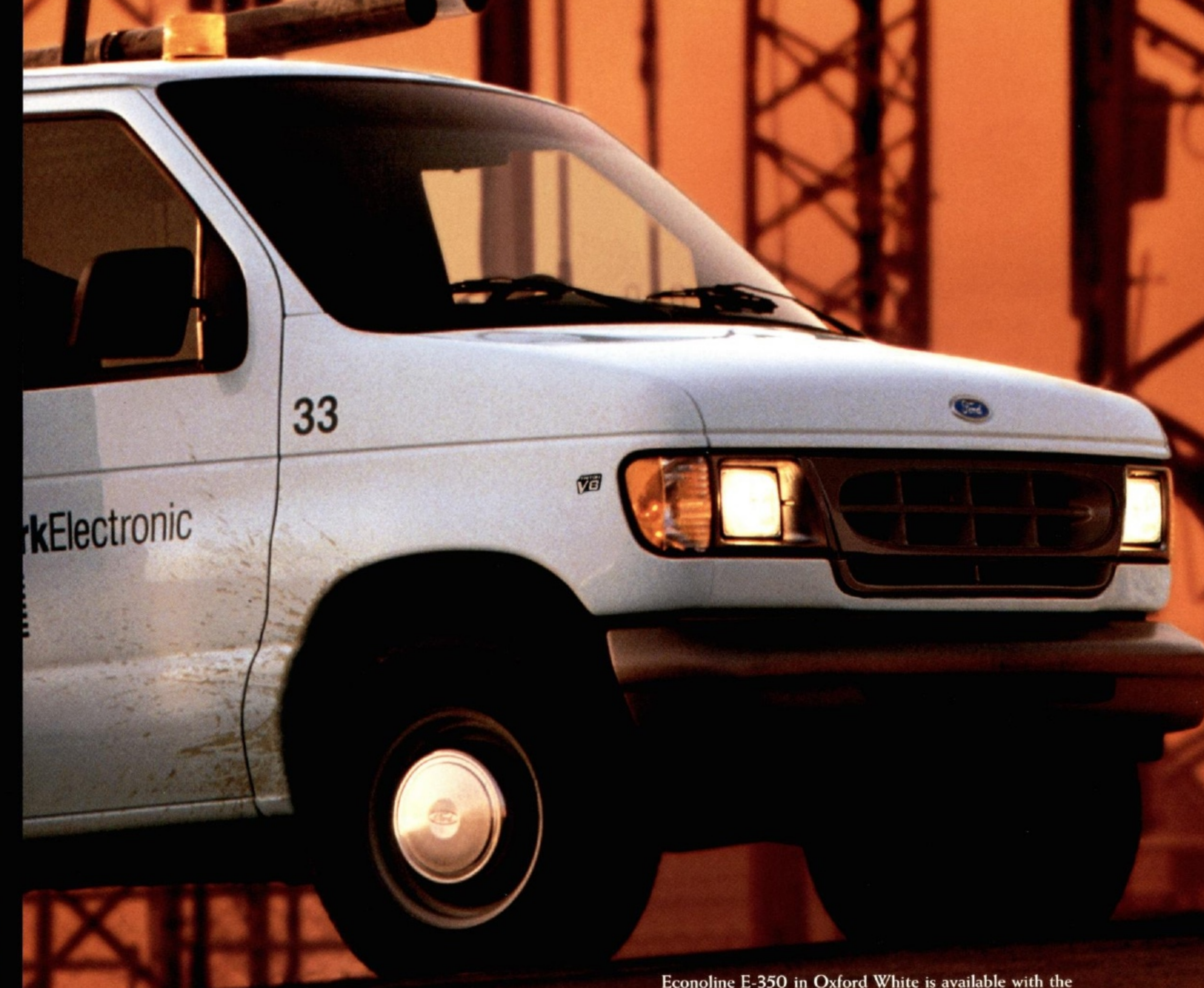
Econoline E-350 in Oxford White is available with the natural-gas-powered 5.4L Triton V8.
