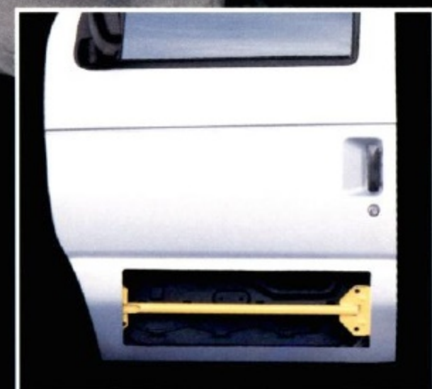
Side door intrusion beams are integral components of Econoline's strong occupant protection system.
