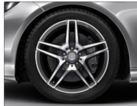
18" AMG 5-twin-spoke alloy wheels with 245/40 R18 front and 265/35 R18 rear tyres (standard on AMG Sport, code 660)
