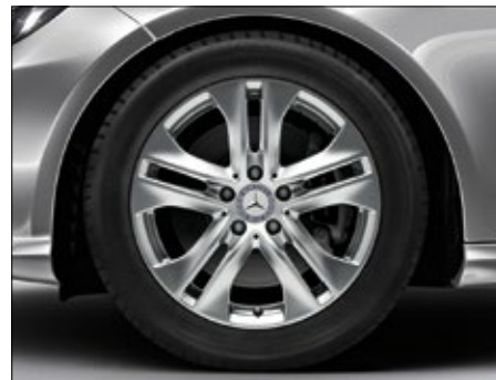
17" 5-twin-spoke alloy wheels with 245/45 R17 tyres (no-cost option on SE, code R11)
