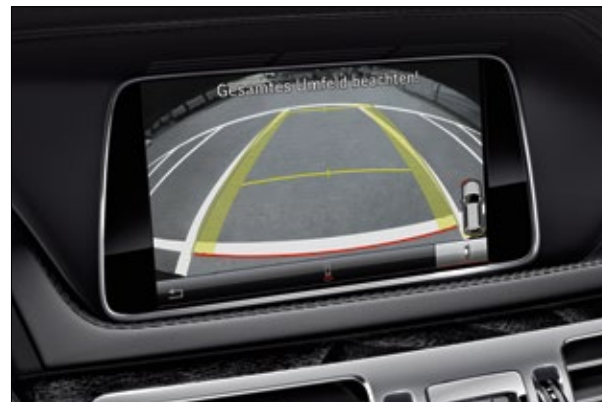
COMAND Online shows the area immediately behind the car when reversing the E-Class
