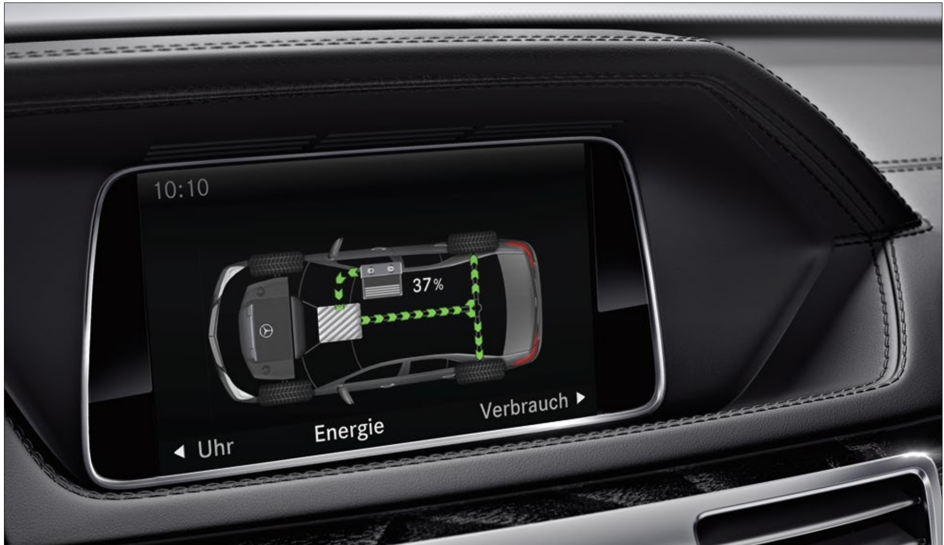
The central display provides information about the current energy flow and the battery's charging status
