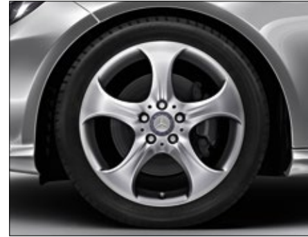
18" 5-spoke alloy wheels with 245/40 R18 front and 265/35 R18 rear tyres (optional on SE, code R08)
