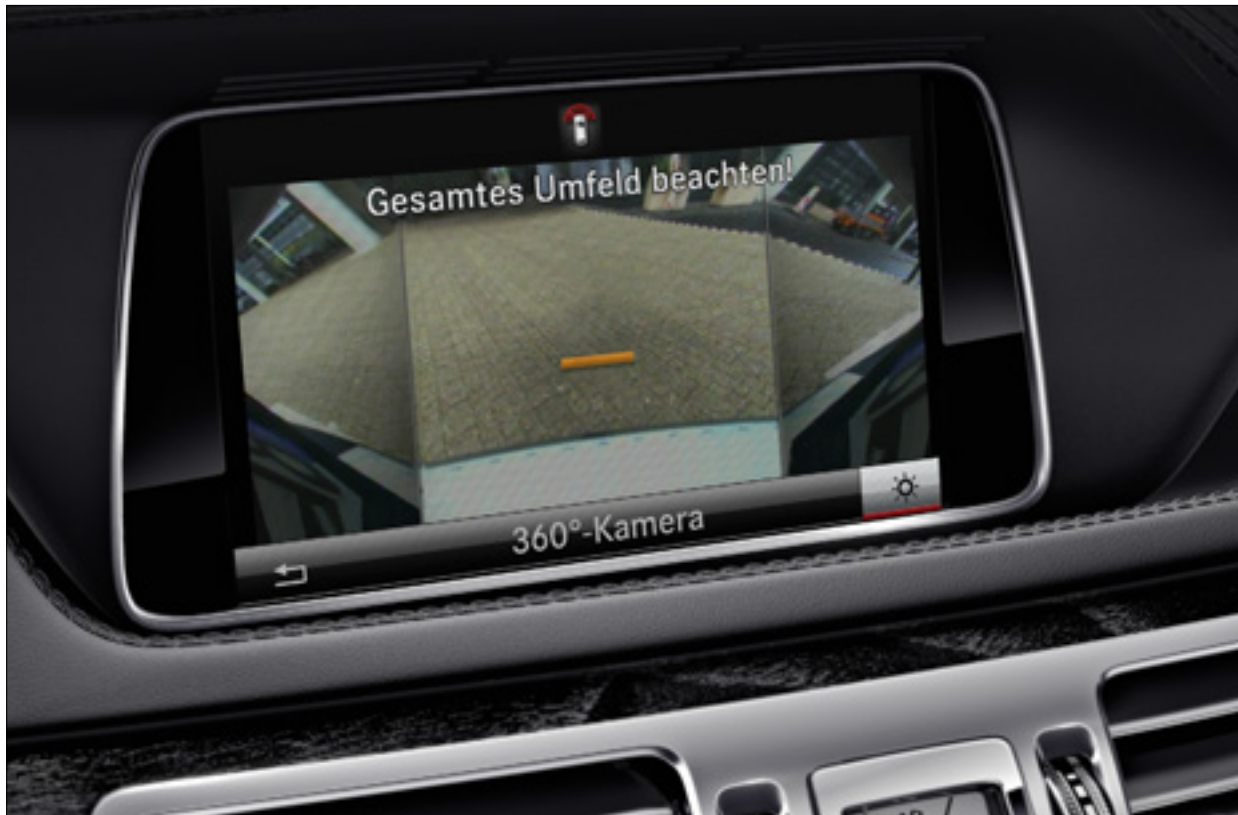
Using four individual cameras the 360° camera presents a continuous view all around the vehicle
