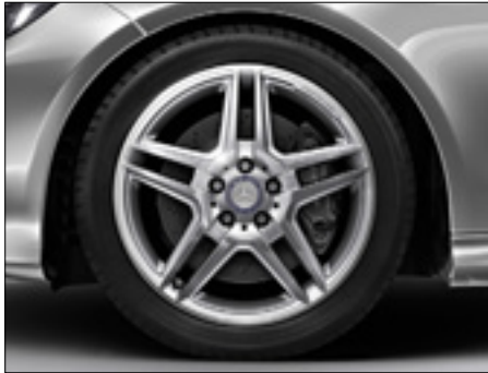
18" AMG 5-twin-spoke alloy wheels with 245/40 R 18 front and 265/35 R 18 rear tyres (optional on AMG Sport, code 795)
