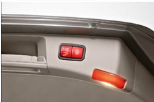
The Easy-Pack tailgate can also be opened and closed in a lower position at the push of a button
