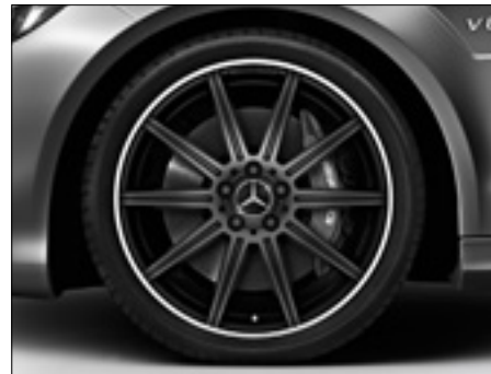
19" AMG 10-spoke alloy wheel painted in matt black, with 255/35 R 19 front and 285/30 R 19 rear tyres (optional on E 63 AMG and E 63 AMG S, code 752)
