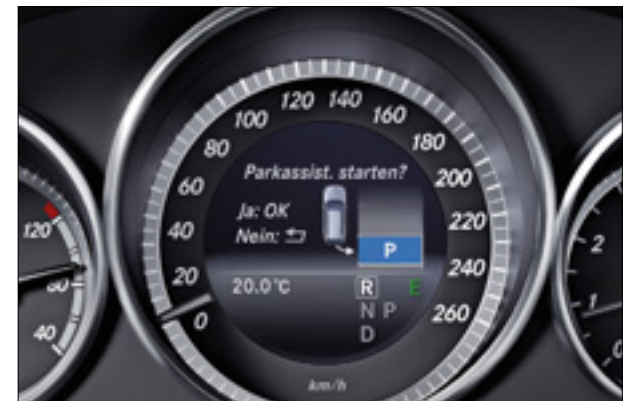
The instrument cluster displays the status of the current parking process
