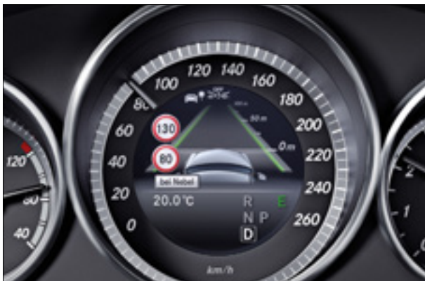
COMAND Online and the multi-function display in the instrument cluster show vital Speed Limit Assist and Traffic Sign Assist information
