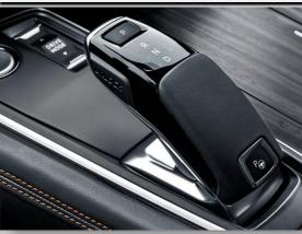
'Electric Impulse' Automatic Gearbox Control
