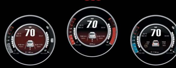
That's why it can feature an on-board 7" TFT digital display which, apart from being uber-cool, is useful for monitoring all the information you could possibly need while driving, like the information from the speedometer, the rev counter, the temperature, the **gear shift indicator** and the trip computer. What's more, everything is perfectly integrated with the **Uconnect™ 5" Radio LIVE**, which let you see the media player, telephone and navigator on the same screen.
