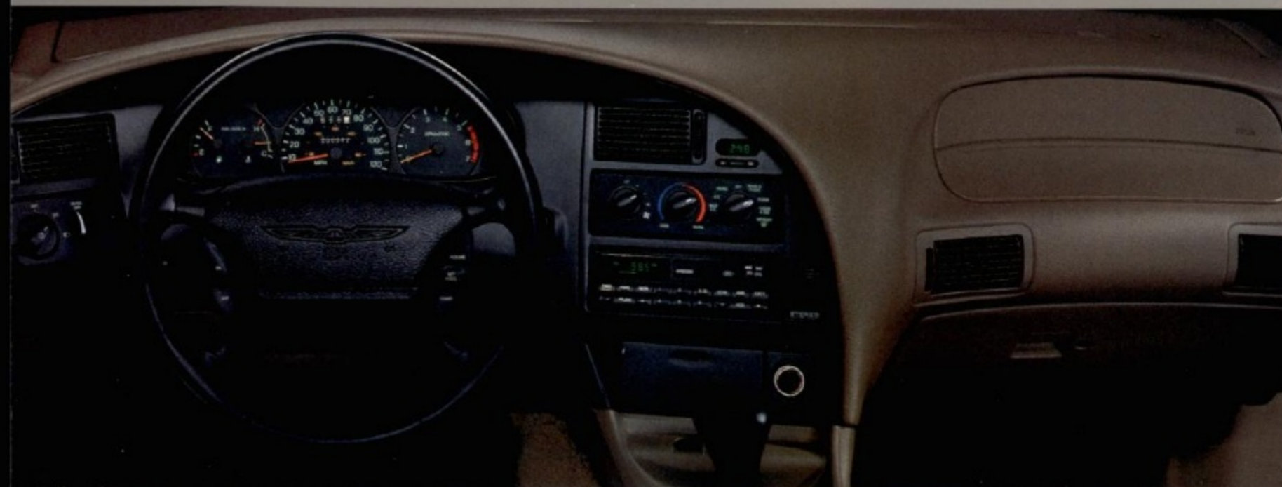
THE NEW PERFORMANCE INSTRUMENT CLUSTER is highly ergonomic and includes a tachometer as well as low fuel level, low washer fluid, low coolant level and door ajar indicators.
