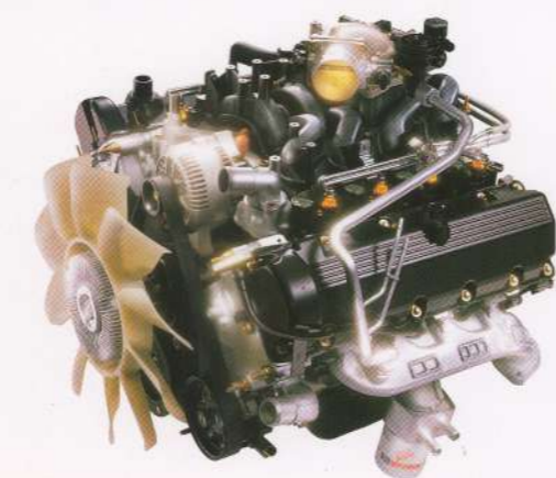
The 5.4L V8 is one of three powerful Triton™ engines available with Econoline. Optional on E-150 and standard with the E-350 Super Duty model, its single-overhead-cam design is equipped with a maintenance-free silent chain drive which eliminates push rods and allows design flexibility for improved horsepower and torque.
