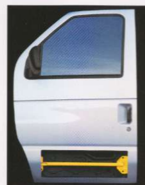
Side door intrusion beams are integral components of Econoline's strong occupant protection system.
