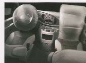
Second Generation airbags are designed to further enhance protection for driver and passenger while also reducing the risk from potential airbag inflation injury.
