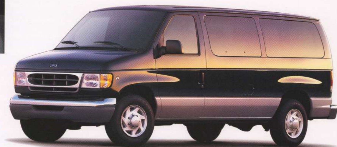
A properly equipped E-350 Super Duty Wagon with the standard 5.4L Triton™ V8 can tow up to 7,000 pounds. (Up to 10,000 lbs. may be towed with the available 6.8L V10.)
