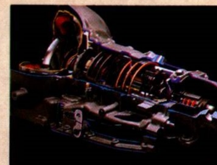
The fourth gear on Mark VII's automatic overdrive transmission is 100% mechanical drive, so there's virtually no slippage.
