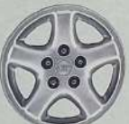
15x7-inch ECCO Cast Aluminum. Available in the Ecco Wheel and Tire Group
