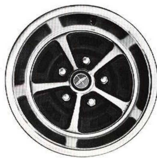
Styled Steel Wheel with Trim Ring (4), Not Available on Cougar XR-7, Optional on all other Models
