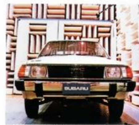
Subaru vehicles are tested in an anechoic chamber to reveal resonances, vibrations and noise emissions.
