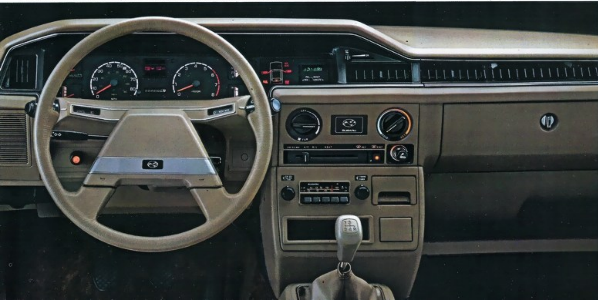
GL 4WD dashboard, Beige, with voltmeter, fuel gauge, speedometer, trip odometer, tachometer, oil pressure gauge, temperature gauge, Telltale Graphic Monitor, quartz digital clock, AM/FM stereo 4-speaker system and optional air conditioning.
