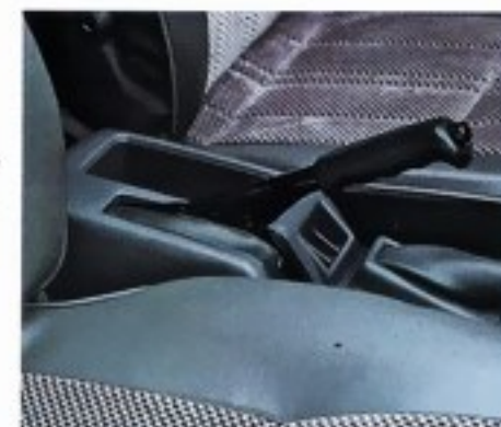
Emergency brake engages the front disc brakes.
