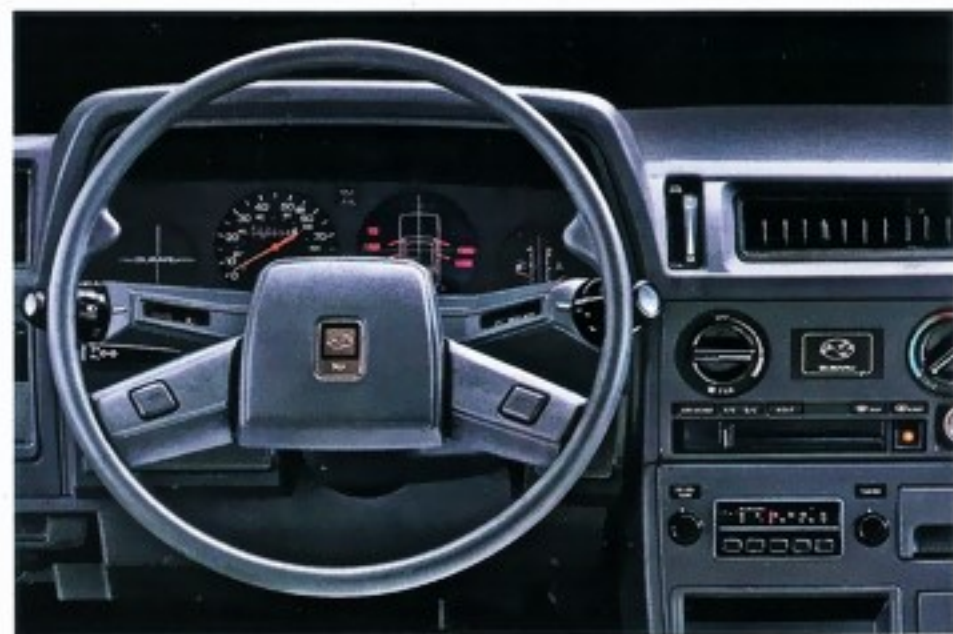
DL dashboard, Gray, with speedometer, alternator and oil pressure warning lights, Telltale Graphic Monitor, fuel gauge, temperature gauge, illuminated switch and control function labels, AM/FM radio and optional air conditioning.
