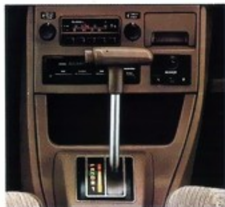
Center console, GL Wagon, with optional automatic transmission, cassette deck, and control for remote electric mirrors.
