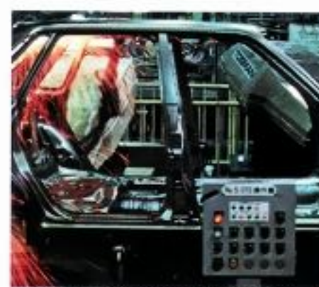
Computer-controlled robots uniformly weld thousands of points to create strong, rattle-free, unitized bodies that meet exacting Subaru standards.
