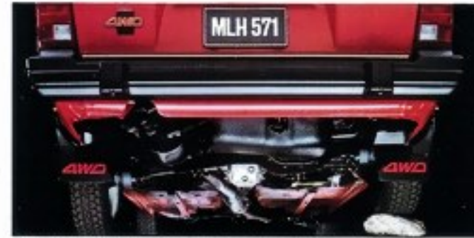
4-wheel fully independent suspension allows each wheel to individually absorb bumps for better handling, traction and comfort.
