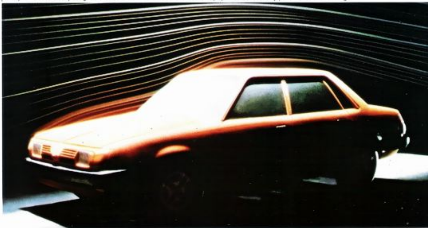
Aerodynamic Subaru body designs are tested in the wind tunnel, and refined to help optimize fuel economy, performance and handling.
