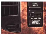
TWILIGHT SENTINEL HEADLAMP CONTROL turns the headlamps on at dusk or the appropriate time when light has faded. Optional, it also delays "lights out" when you have turned the ignition off.
