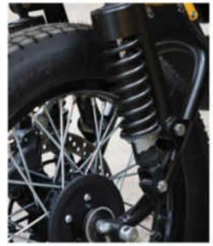
Strong rear suspension thanks to the double-sided swingarm and twin Sachs hydraulic spring shocks
